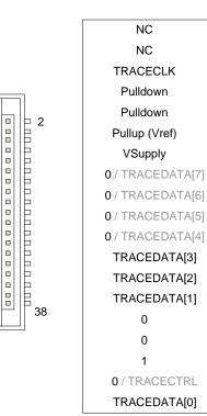
The Mictor connector is still the recommended trace connector for other ARM processors including ARM7, ARM9, Cortex-R and Cortex-A processors, and other applications that require wider trace widths (e.g multiple processors).
