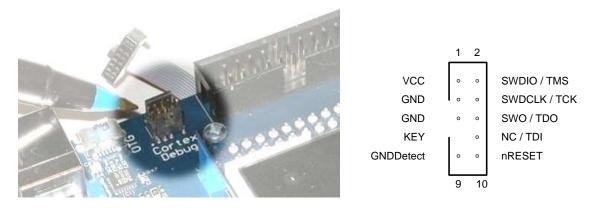
The Cortex Debug Connector supports JTAG debug, Serial Wire debug and Serial Wire Viewer (via SWO connection when Serial Wire debug mode is used) operations.
