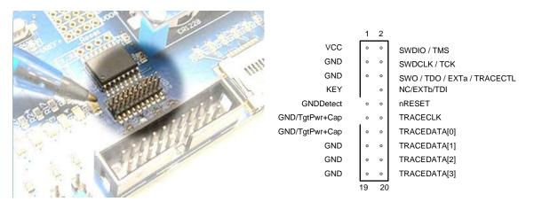
The Cortex Debug+ETM Connector supports JTAG debug, Serial-Wire debug, Serial Wire Viewer (via SWO connection when Serial Wire debug mode is used) and instruction trace operations.
