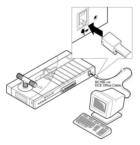
Figure 7- 2 Connecting to the Terminal
