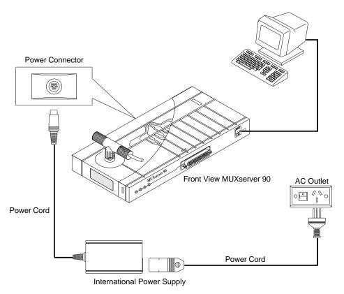
Figure 5- 4 Stand- alone Installation with International Power Supply
