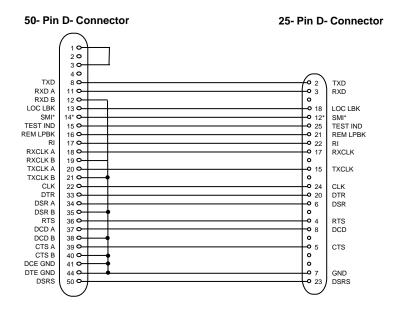
\*The SMI connection between pin 14 on the 50- pin D- connector and pin 12 on the 25- pin D- connector is not present in the BC19V- 02 or the BC19D- 02, but applies only to the BC23V- 02. (SMI signal is not required for the MUXserver 90.)
