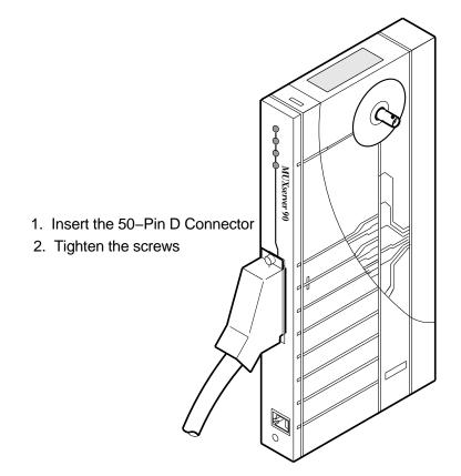
Figure 7-5 Connecting an Adapter Cable to an Extension Cable
