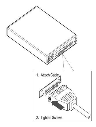
Figure 7- 7 Connecting Adapter Cable, V24/RS- 232- C Adapter, and Extension Cable
