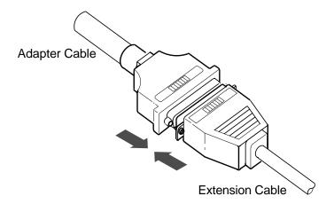
Figure 7-6 Connecting to the Modem
